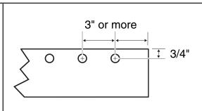
Figure 2. Drilled hole dimensions.
